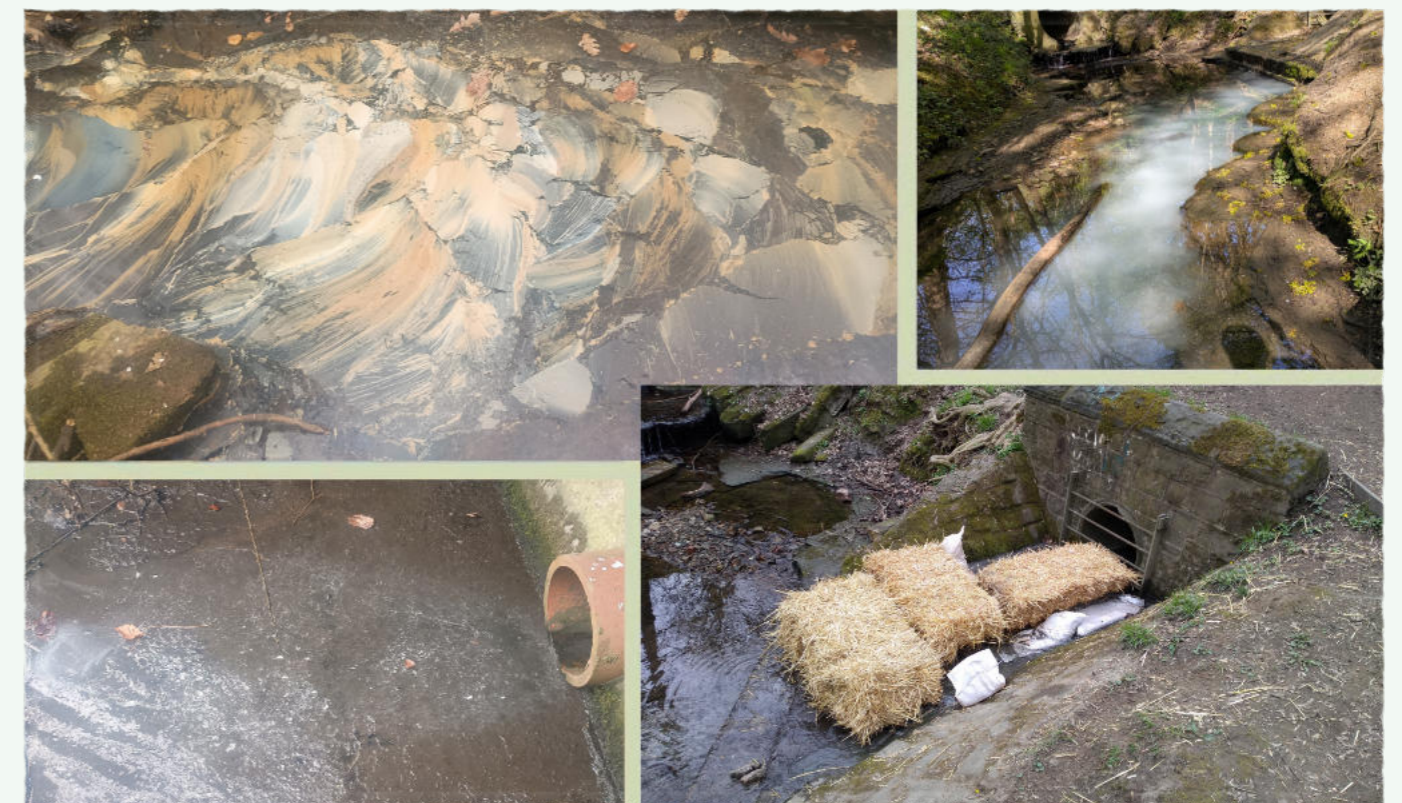
Figure 7, Pollution from misconnected plumbing in the Gledhow Valley
